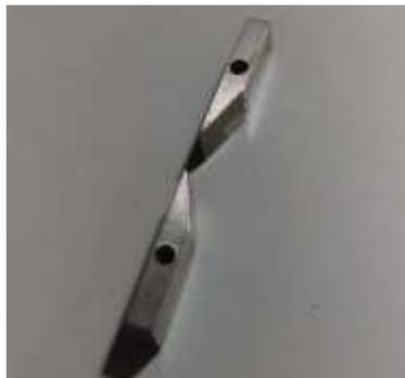
Figure 17. A pair of electrodes made of aluminum that simulate the plasma electrode.
