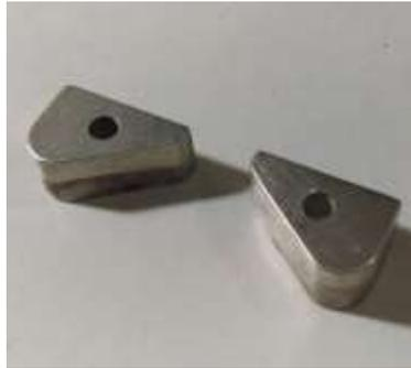
Figure 16. A pair of electrodes made of aluminum that simulate the extraction electrode.
