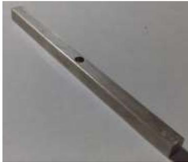
Figure 19. Electrode made of aluminum that simulates the saturation electrode. Source: author.
